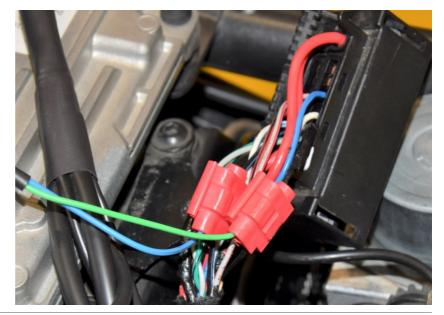
Lift up the fuel tank and locate the Clutch switch connector on the right side.
