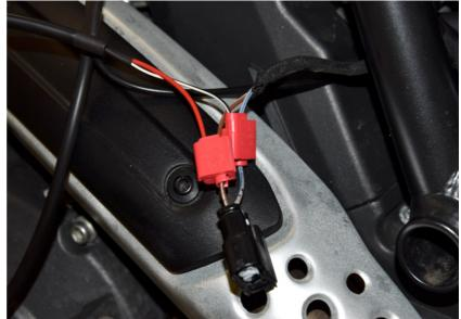
Splice the ARA White wire to the Gray/Green wire at the vertical coil connector.
