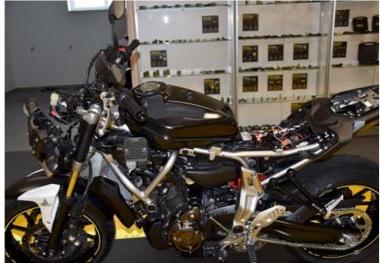
Locate the ignition coil connectors below the fuel tank.
