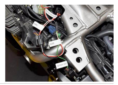
Connect the ARA black wire terminal to the battery negative.
