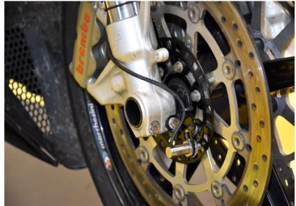
Mount the supplied disk and wheel speed sensor at the rear wheel.
