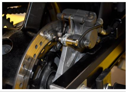
Connect the 3-pole rear wheel speed sensor connector to the ARA wiring.
