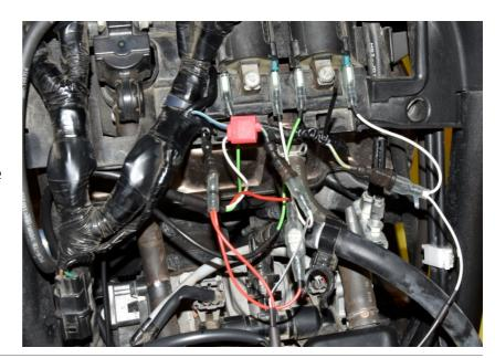
Locate the ABS ECU connector at the rear of the bike.
