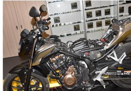
On this bike the ARA used together with the iQSE quickshifter. The iQSE plugs should always be the last in the chain i.e. connected directly to the ignition coil plugs.
