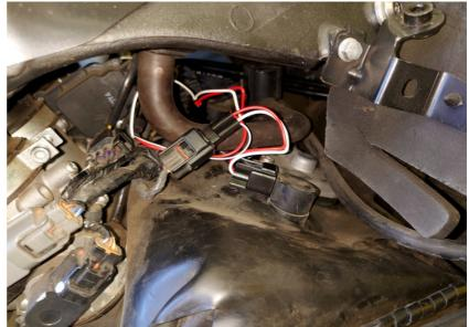
Connect the ARA Black wire terminal to the chassis ground.
