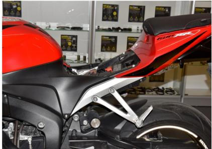
Remove the side fairings and plastic covers around the fuel tank.
