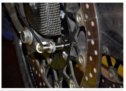
Connect the 3-pole sensor connector to the ARA wiring.
