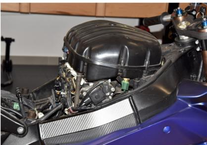
Remove the airbox to gain access to the ignition coil connectors.
