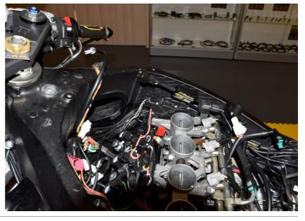
Plug the ARA connectors in-line with the ignition coil connectors.
