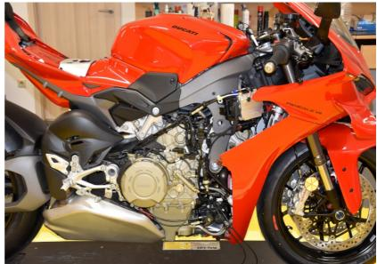
Locate and unplug the exhaust servo motor connectors.
