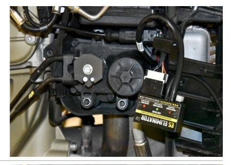
Locate the ABS connector over the exhaust servo motor.
