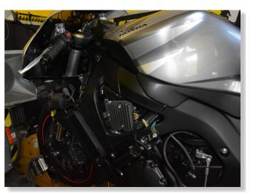
CONNECT DS-SERIES CONNECTOR TO DIAGNOSTIC SYSTEM CONNECTOR.
