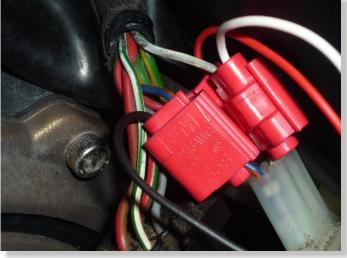
CONNECT GPX GREEN WIRE TO BLUE/YELLOW WIRE OF CAMSHAFT POSITION SENSOR CONNECTOR. (BLACK, 3-POLE CONNECTOR ON CYLINDER HEAD AT THE LEFT)
