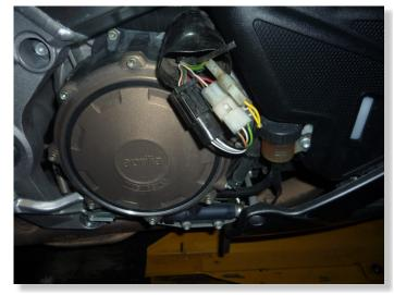
REMOVE THE MAIN SEAT. LIFT UP OR REMOVE THE FUEL TANK. LOCATE THE SPEED SENSOR CONNECTOR. ROUTE THE GPX CABLE THROUGH THE TOP OPENING OF THE DUST BOOT
