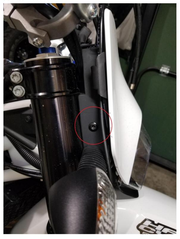
On the Left side remove the two remaining screws, one above and one below the turn indicator. Shown below in the circles.
