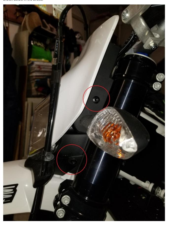
Pull the headlight assembly away from the motorcycle and disconnect the headlight connector, circled below.
