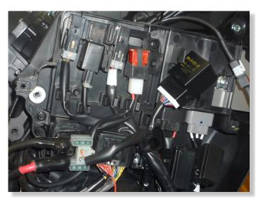
REMOVE THE FAIRINGS FROM RIGHT SIDE. REMOVE THE RELAY HOLDER.
