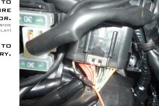
CONNECT GPX RED WIRE TO BROWN WIRE AT THE WIRE DISTRIBUTOR CONNECTOR. (BLACK CONNECTOR AT RIGHT SIDE NEAR MAIN RELAY)
