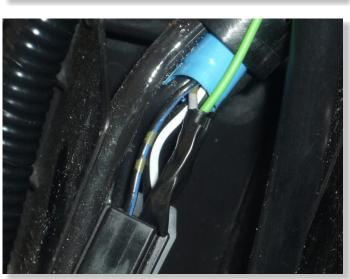
CONNECT GPX GREEN WIRE TO GRAY WIRE OF CRANKSHAFT POSITION SENSOR CONNECTOR. (BLACK, 2-POLE CONNECTOR AT RIGHT SIDE)
