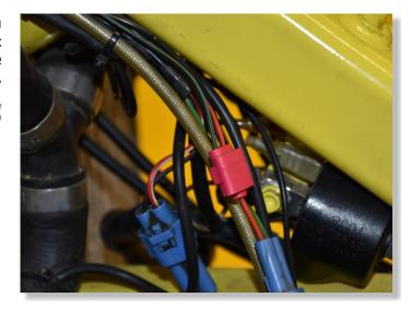
CONNECT THE 3-POLE SENSOR CONNECTOR TO THE GPX WIRING HARNESS CONNECTOR.
