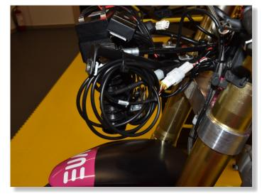
CONNECT THE 3-POLE SENSOR CONNECTOR TO THE GPX WIRING HARNESS CONNECTOR AND COIL UP THE EXCESS LENGTH.
