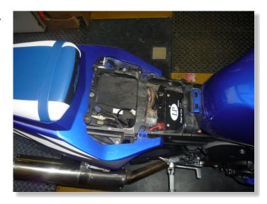
LIFT UP OR REMOVE THE FUEL TANK.
