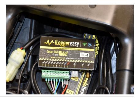
Splice the iLE Blue VSS wire to the Pink/Green wire of the speed sensor connector.
