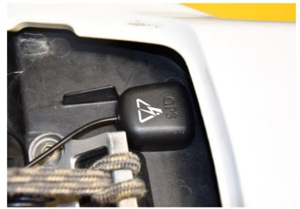
Typical position for the iLE module.
