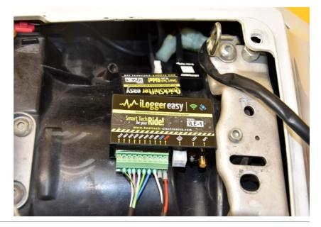
Splice the iLE Blue VSS wire to the Pink wire of the speed sensor connector.
