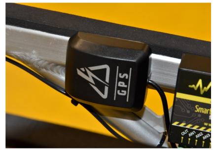
Typical position for the iLE module.
