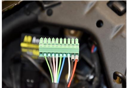
Connect the green terminal block to the iLE modul.
