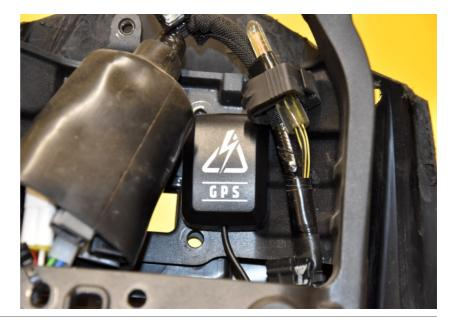
Typical position for the iLE module.
