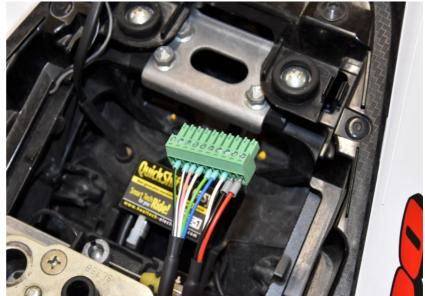
If the iLE is used together with the iQSE quickshifter, plug the iLE-H-iQSE connectors in-line with the 4-pole iQSE connectors, then connect the Red, Black and White wires to the green terminal block.
