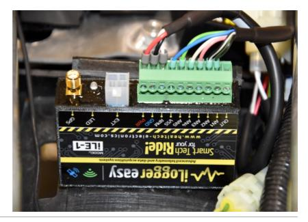
Splice the iLE Blue VSS wire to the Black wire of the speed sensor connector.
