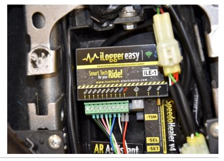
Splice the iLE Blue VSS wire to the White/Yellow wire of the ABS connector.
