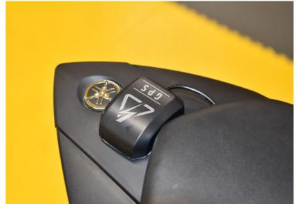
Typical position for the iLE module.
