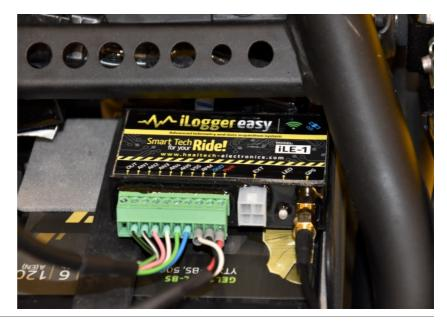
Splice the iLE Blue VSS wire to the White wire of the ECU connector.
