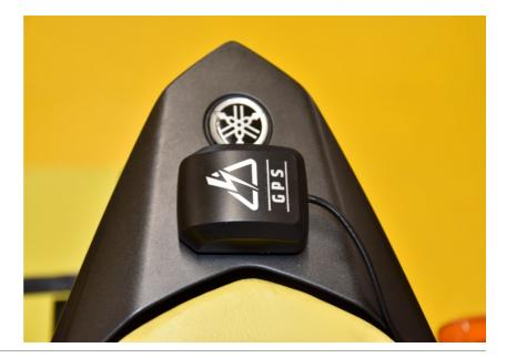
Typical position for the iLE module.
