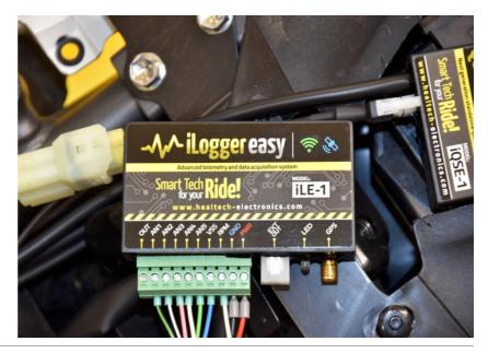
Splice the iLE Blue VSS wire to the White/Yellow wire of the ABS connector.
