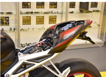
Plug the MM connector to the OBD connector.
