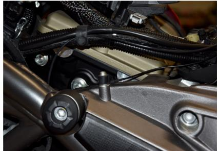
Replace the bolt of the shift lever by the supplied bolt and add the spacer, washers and sensor exactly as shown on this photo.
