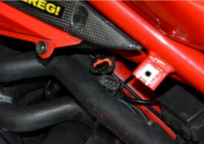
Plug the QSH connectors in-line with the ignition coil connectors of the rear cylinder.
