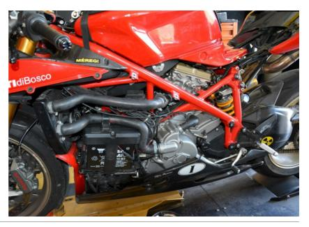
Plug the QSH connectors in-line with the ignition coil connectors of the front cylinder.
