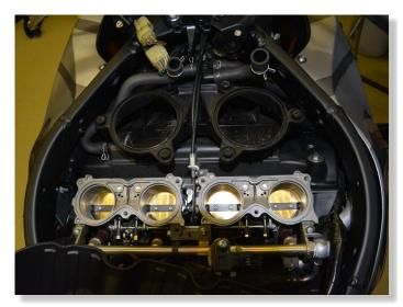
REMOVE THE AIR INTAKE BELOW THE AIRBOX.
