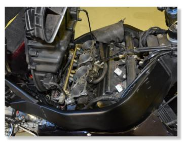
PLUG QSH CONNECTORS IN-LINE WITH THE IGNITION COIL CONNECTORS. (BLACK, 2-POLE CONNECTORS BELOW AIR INTAKE)
