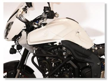
REMOVE THE FUEL TANK AND THE AIRBOX.
