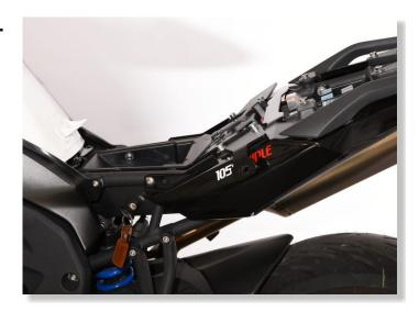
REMOVE THE FUEL TANK COVERS AND THE SIDE FAIRINGS.
