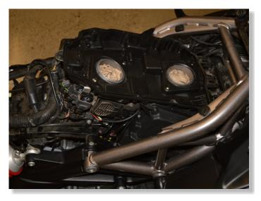
CONNECT THE QSH CONNECTORS IN-LINE WITH THE IGNITION COIL CONNECTORS ON THE LEFT SIDE. (BLACK, 3-POLE CONNECTORS)
