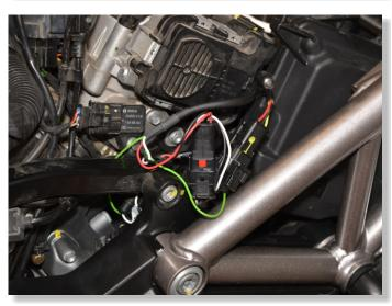
CONNECT THE QSH CONNECTORS IN-LINE WITH THE IGNITION COIL CONNECTORS ON THE RIGHT SIDE. (BLACK, 3-POLE CONNECTORS)
