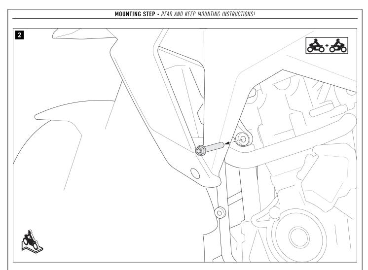
Push the side panel a little to the side to be able to remove the original screw.
