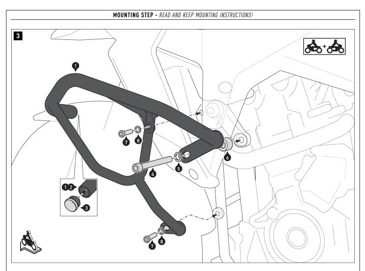
Insert the plastic plugs (3) into the openings on the crash bars (1) and (2) as shown in the detail drawing.
